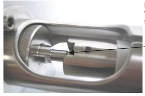
Bring together the handwheel and the cutter drum. When merging the two parts, please pay attention that they meet the <u>slots.</u>
