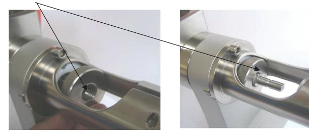
Insert the handwheel (3) into the body (1).
